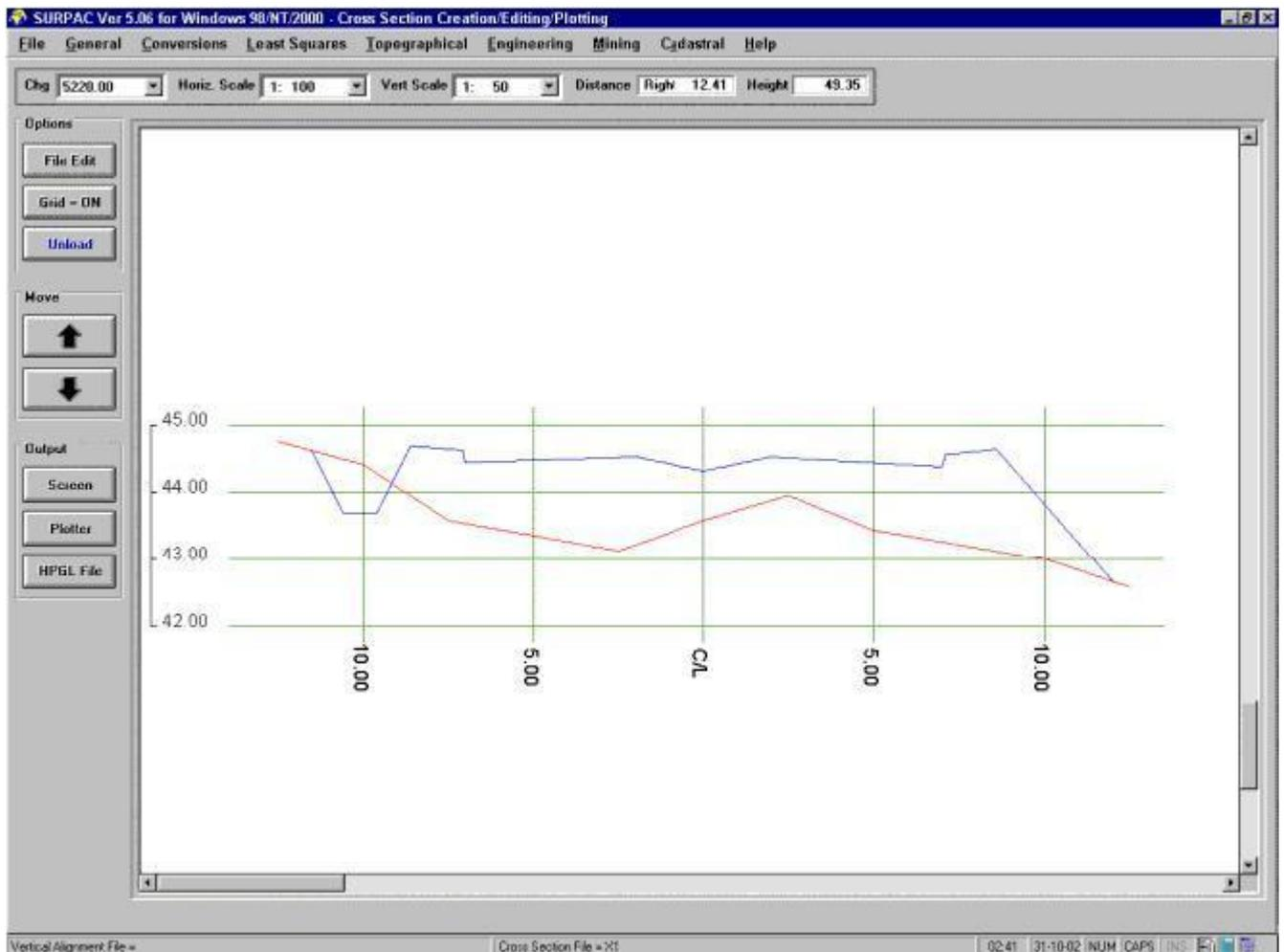
The Cross Section Plotting Programme, showing both Ground and Design Sections
